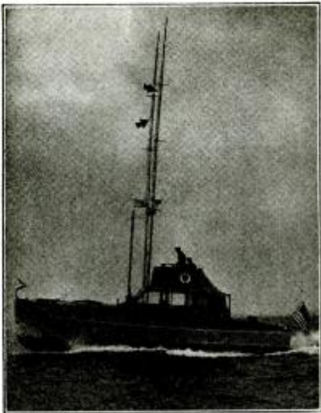
Fig. 2. Corair II , a sport fishing cruiser owned by Lt. Everett Walsh of the South Shore (L. I., N. Y.) Power Squadron is a typical installation in which the tall outrigger poles support aerial wires (arrows) which run their entire length down to the deck below.
